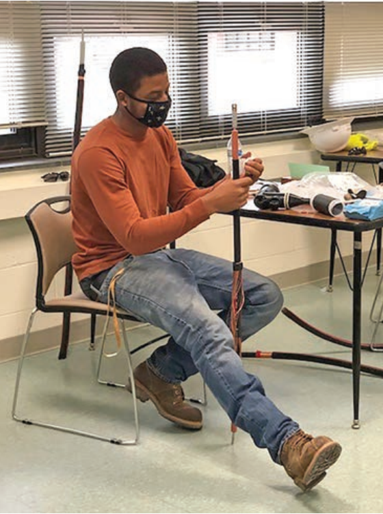
Students at Durham Tech are learning how to terminate high voltage cables by making up cable ends and outfitting with elbow connections.
